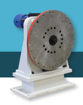
Motion Index Drives' Weld Positioners utilize the TR series headstock / tailstock trunnion sets, on a high precision (less than 1 arc minute) planetary gear system. It is mounted in a vertical position complete with mounting plates and is ideal for moving large masses with smaller units, minimizing your equipment's footprint on the floor. Weld Positioners can be ordered with tailstock supports and one-piece base weldments.
