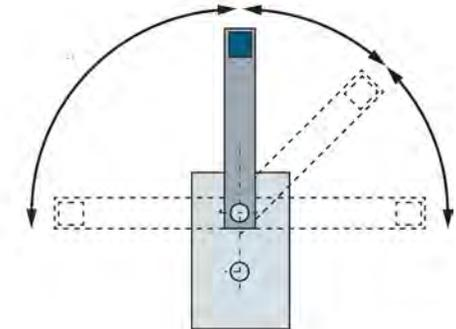
Transducer of rotations in horizontal movement
